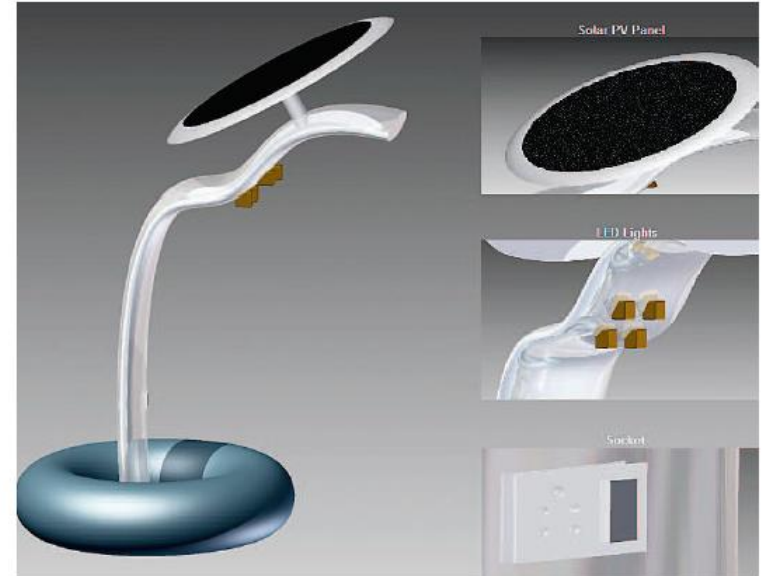
Above: A study lamp that could absorb solar rays through photovoltaic panels installed on the upper side of the lamp
